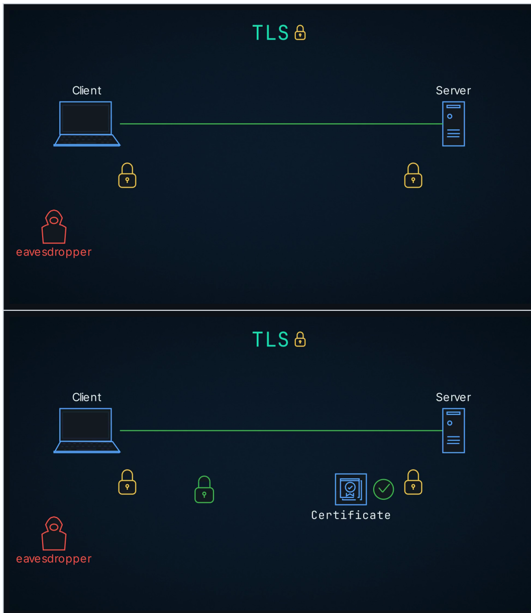
the Diffie-Hellman exchange and certificate check; the padlock closing once the secret is agreed.
